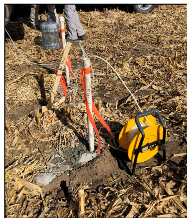
Development/sampling of temporary PM wells: EW7-PM25A (shallow) and PM25B (shallow intermediate)
