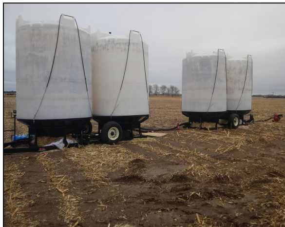
Two 6,000-gallon trailer tanks w/ mixed amendment and firefighter pumps (facing east)
