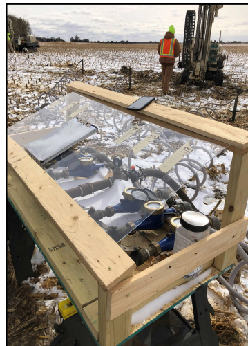
Subsurface injection and manifold system at EW7-T16, points 1-6 (facing southwest).
