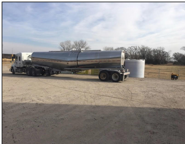
Bulk delivery of amendment (Westway). Off loaded into 4 x 3000-gallon tanks at GWTF. Each delivery approximately 45,000 lbs / 4,500 gal. (facing east)
