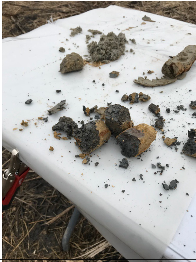
Photo 1-Clay similar in color to the “Blue Clay” typically encountered at the base of the LGIA was encountered at 20B-MW02 from 8.5 to 9 ft bgs.
