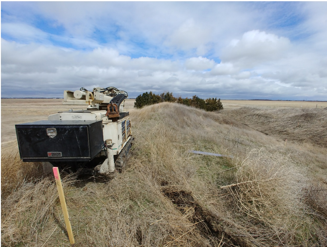
Photo 2 – The 6600 Geoprobe that was parked on top of the eastern stockpile at the end of the day. The driller felt confident in the improved site conditions to mobilize the unit to the top of the stockpile.
