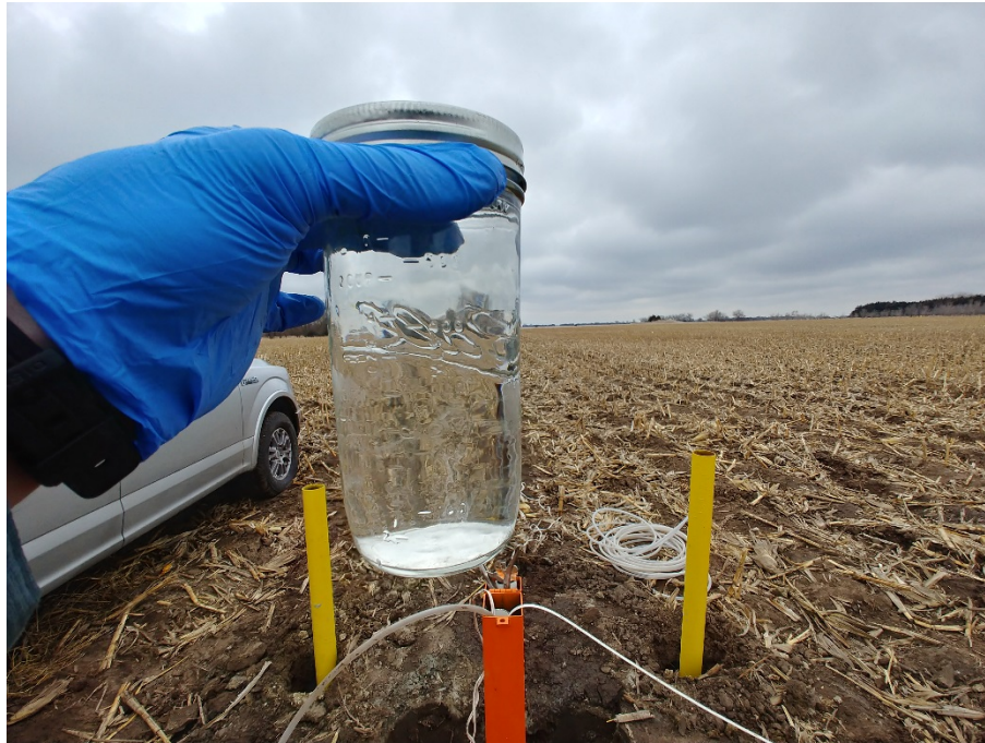
Photo 1 – Water at 21C-LGIA-MW04 after well development and prior to surface completion.
