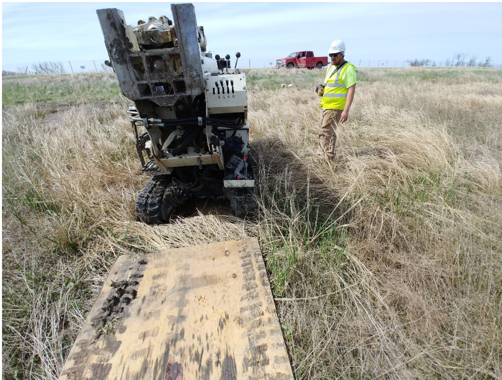
Photo 2 – The DPT handler maneuvering the 6600 Geoprobe rig across the plywood to keep from sinking into the soft ground.
