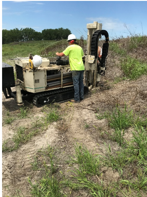
Photo 1: This DPT Rig is used to advance soil sampling cores and groundwater sampling screens.
