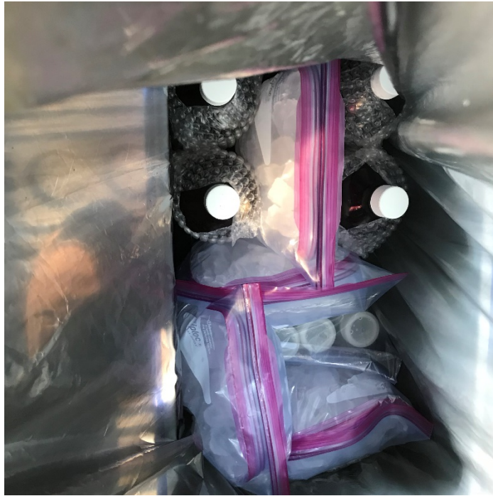
Photo 1: Samples are situated in the cooler so that all bottles are in contact with double-bagged ice-bags.
