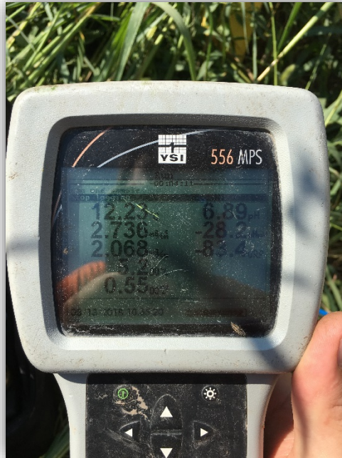
Photo 1: A YSI-556 water quality meter displays the readings that are recorded during purging.
