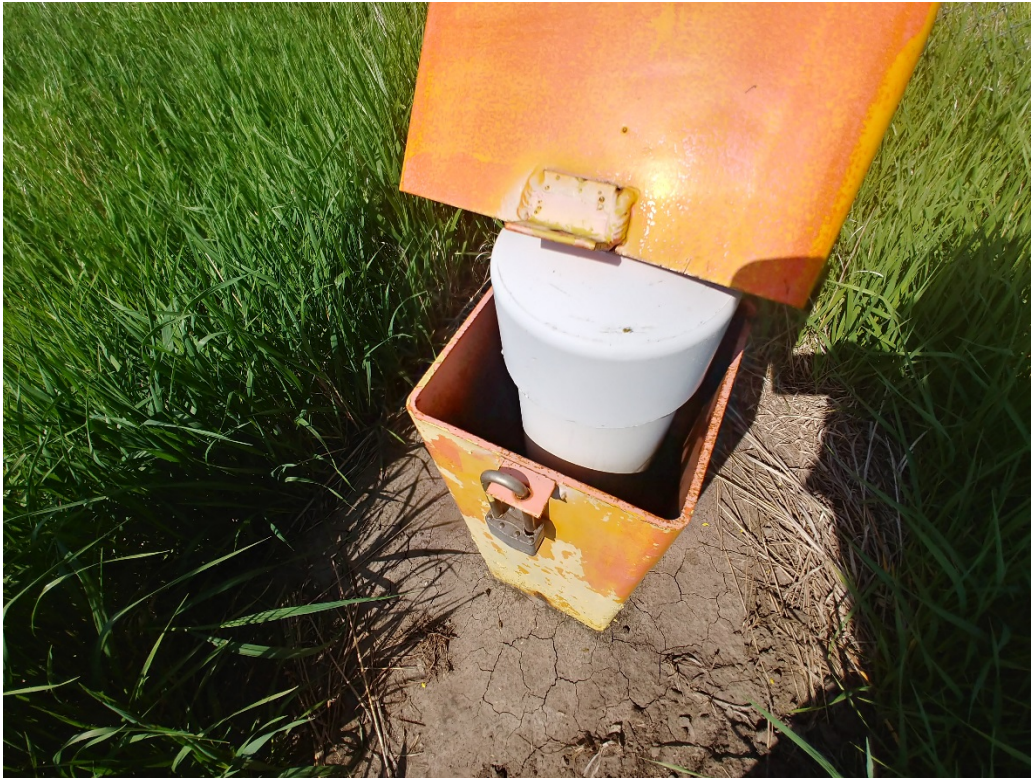
Photo 5 – BGMW02 being unable to close due to the height of the PVC casing.
