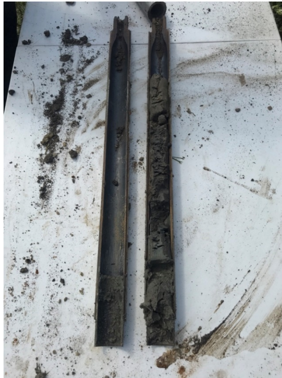
Photo 2: Monitoring well 20B-UGIA-MW10 was screened from 10-20 ft bgs. This split-spoon sample collected from 10.5-12.5 ft bgs illustrates that the clay/sand interface is 12ft below the ground surface at this location. Sand can be seen at the bottom portion of the spoon.
