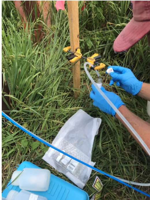
Photo 1: Vials for VOC analysis are tilted at an angle when filled to minimize volatilization of potential contaminants.
