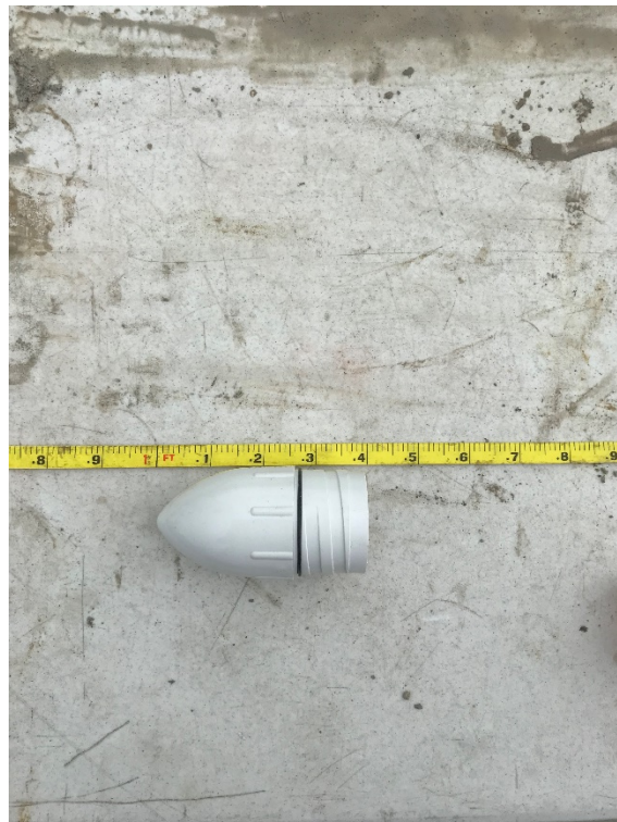
Photo 2: The cap that seals the bottom of the PVC well casing adds 2.5 inches to the total well depth. All wells installed during this 2018 project have a 2.5 inch cap beneath 10 ft of schedule 40, 2" PVC screen.
