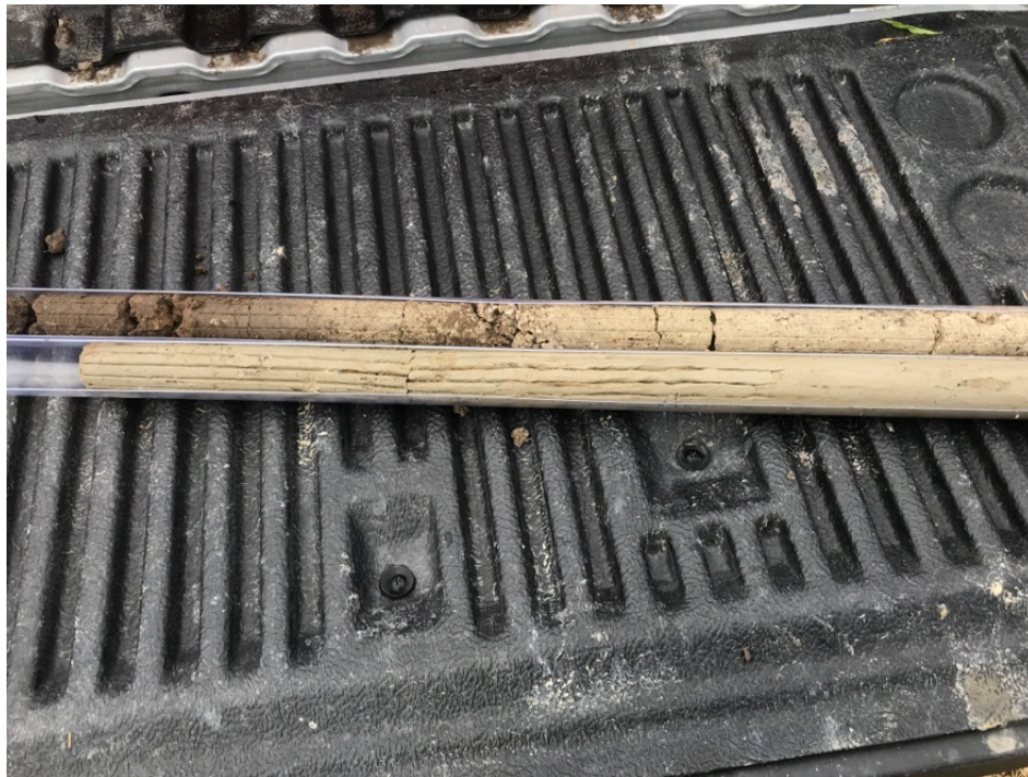
Photo 2: The soil boring collected from Tract 20B extended from the ground surface to 8 ft bgs. The opened soil sleeve can be seen in this photo.
