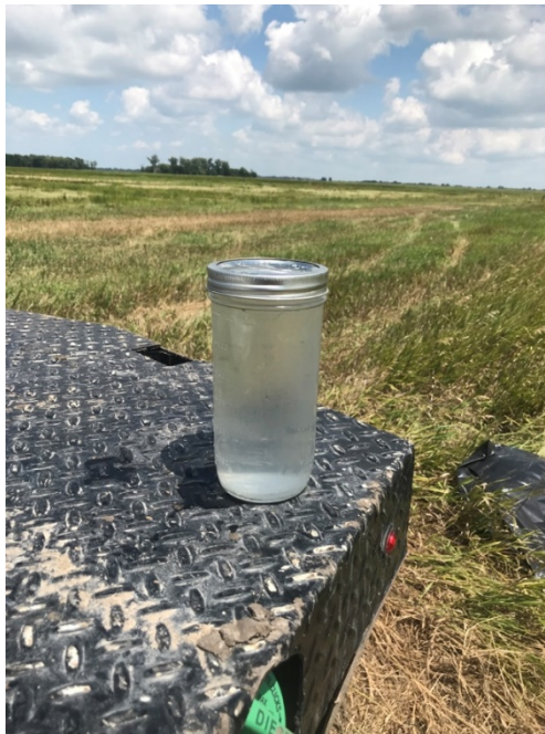
Photo 1: During MW development, once the water quality parameters equilibrate, a photo of the water in a clear jar is taken for record.
