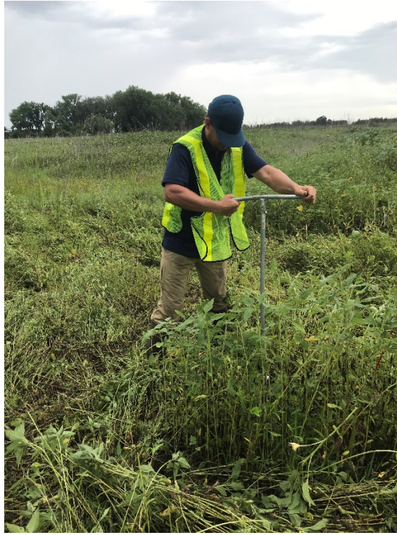
Photo 1: Tip four feet of the borehole for monitoring well 20B-UGIA-MW09 was hand augered and scanned with a Schonstedt.
