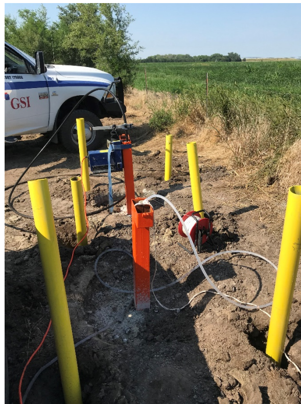
Photo 2: The wells were “surged” by pulling and pushing the pump/tubing up and down throughout the screened interval until water became visibly clear through the tubing, at which point water quality readings began to be collected.
