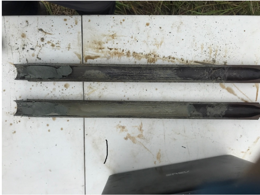
Photo 1: Split spoon collected from 38.5 to 40.5 in the borehole of monitoring well 19C-LGIA-MW07 contained the “Blue Clay” of the Fullerton Formation.
