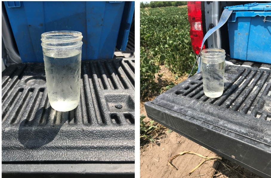
Photo 2: Water from monitoring wells 21B-BPA-UGIA-MW11 (Left) and 21B-DS-LGIA-MW13 (Right) at the end of development is shown above.
