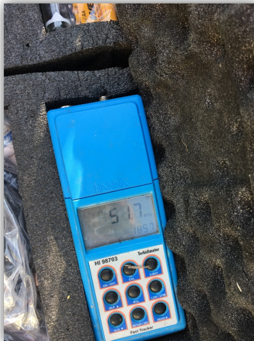
Photo 2: A Hanna Turbidity Meter is used to measure the turbidity of the water throughout purging.
