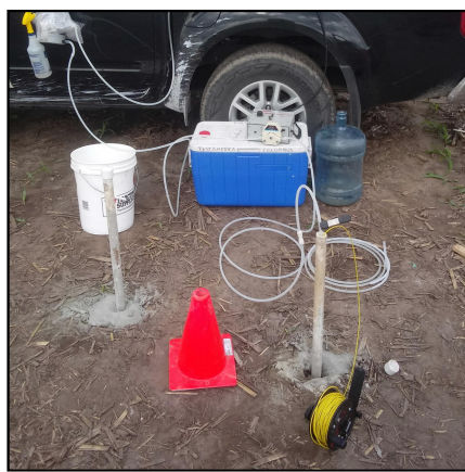
Development and sample purging of EW7-PM24B.
