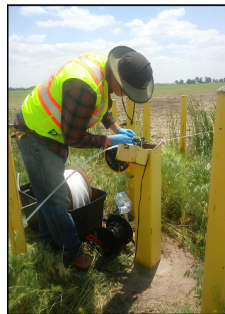
Groundwater purge setup at OU1 off-post monitoring well NW082R (facing south).
