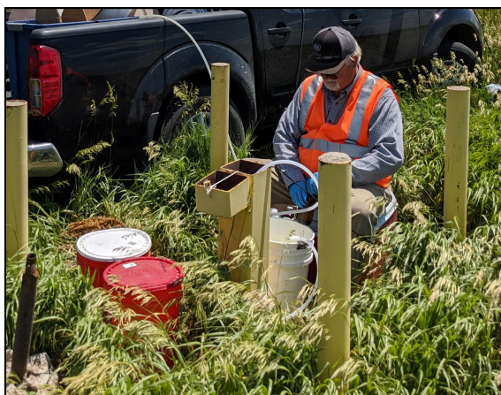
Sample collection at OU1 piezometer PZ017R (facing east).
