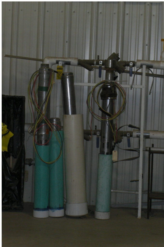
Photo 16 Date: July 31, 2014 Site: CHAAP Description: Removed well pumps in GWTP.
