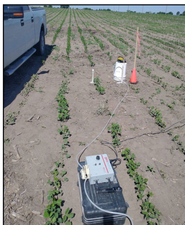
Development and purging of PM temp. wells EW7-PM25A/B (facing east)
