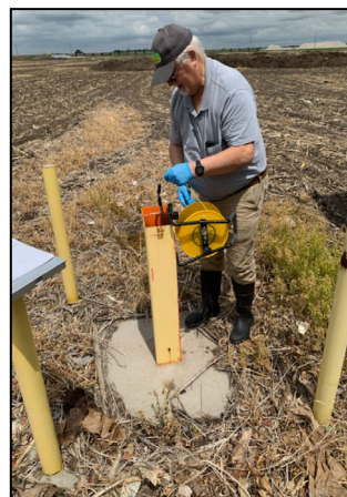
Water level measurement at monitoring well G0093 in LL1 (facing north).
