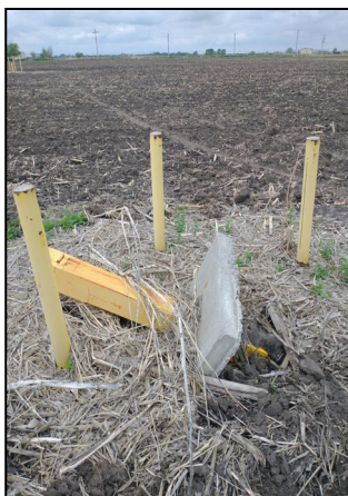
Damaged monitoring well G0120 in LL2 (facing east).
